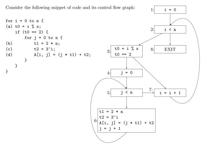
**5.** [6 points]: Draw the dominator tree for your control flow graph. Each node should correspond to a basic block in your control flow graph. Label each node with the corresponding label from the control flow graph.
