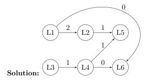
10. [10 points]: Use your dependence DAG to complete the following schedule. Fill in the schedule diagram with the remaining instructions. Note that L3 is scheduled on the ALU because it loads an immediate value into a register and does not access memory.
